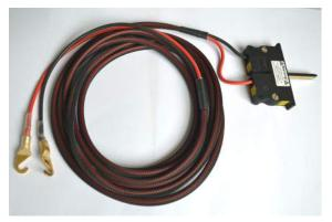
This special test probe allows the connection of current measurement device or a shunt. The AWG 13 (2.5 mm2) connection cable has a length of 118.11 inch (3 meters). The test probe is built with gold-plated C-hook terminals. It is available in an unkeyed version or in a keyed version. Both versions work with all modules of the DOC. Insertion is possible in both directions, so the user has to take care to insert the probe correctly for the intended measurement. The unkeyed version
