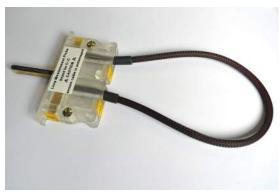
The Loop Measurement Probe serves to redirect the circuit from the drawout case through a cable loop, where it can safely be measured with a clamp-on meter. It is available in an unkeyed version or in a keyed version. Both versions work with all modules of the DOC. Insertion is possible in both directions, so the user has to take care to insert the probe correctly for the intended measurement. The unkeyed version also works in
